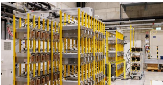
MMC in 200m 2 medium voltage lab © Daniel Karmann / Fraunhofer IISB
